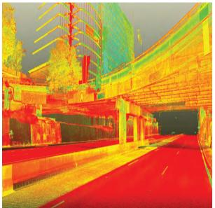
Laser scans of the underside, abutment, top and features of 5 bridge structures along Warringah Freeway. Our Scanning and Aerial Survey Manager generated point cloud from scanner and created a very accurate 3D model with <5mm tolerance as well as establishing a control network for future construction works.
