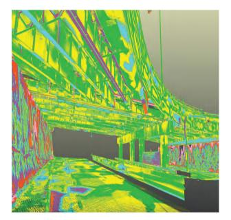
Heatmap generated using Leica 3DRe-shaper to check the accuracy of the 3D model vs point cloud from the scanner. Green signifies that the model is within +5mm accuracy, yellow within -5mm, while the other colours are within +/-10mm.
