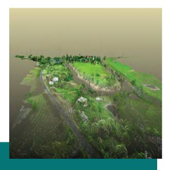
A combination of Aerial and LiDAR Bathymetric & Topographic surveys. This project took 14 days, including reconnaissance and setting out control. 18 single-grid flights at 80m AGL are flown along the river path.
